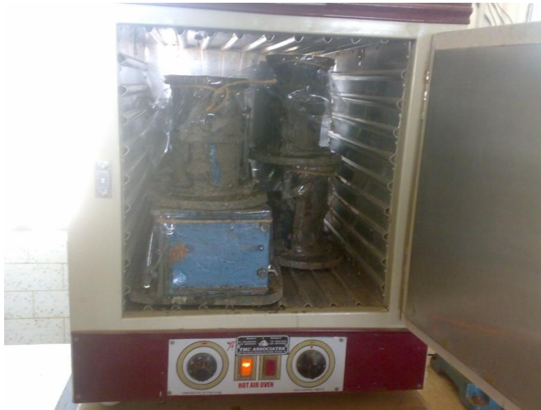
Curing of Geopolymer concrete specimens in the oven
