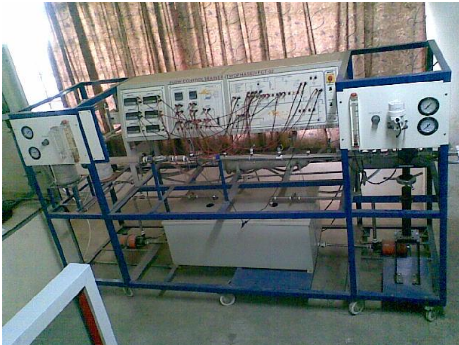
Experimental set up for two-phase flow studies across control valve and pipe in series
